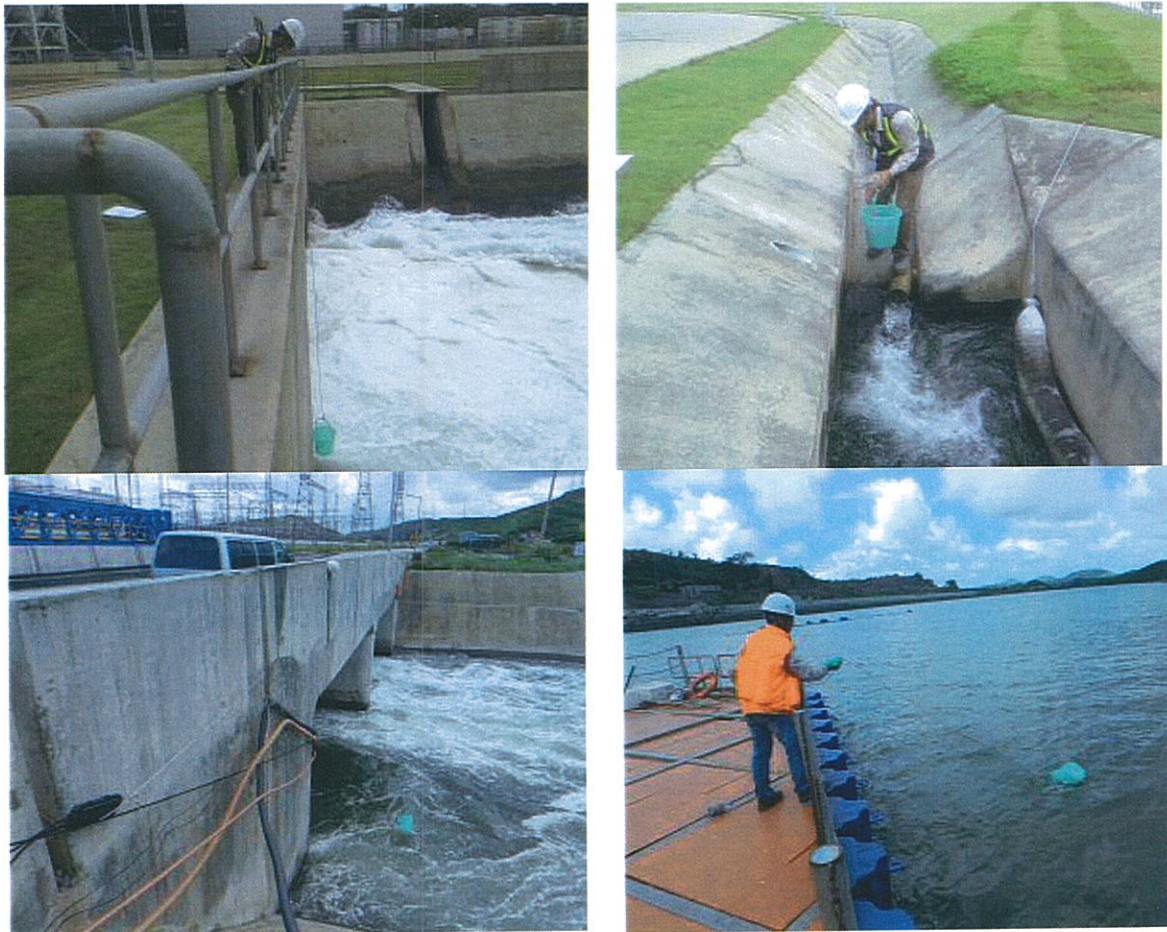
Figure 4.2. Sampling water in Mong Duong 2 thermal power plant
