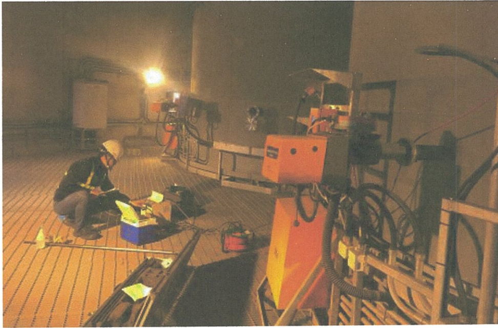
Figure 3.4. Air emission sampling
