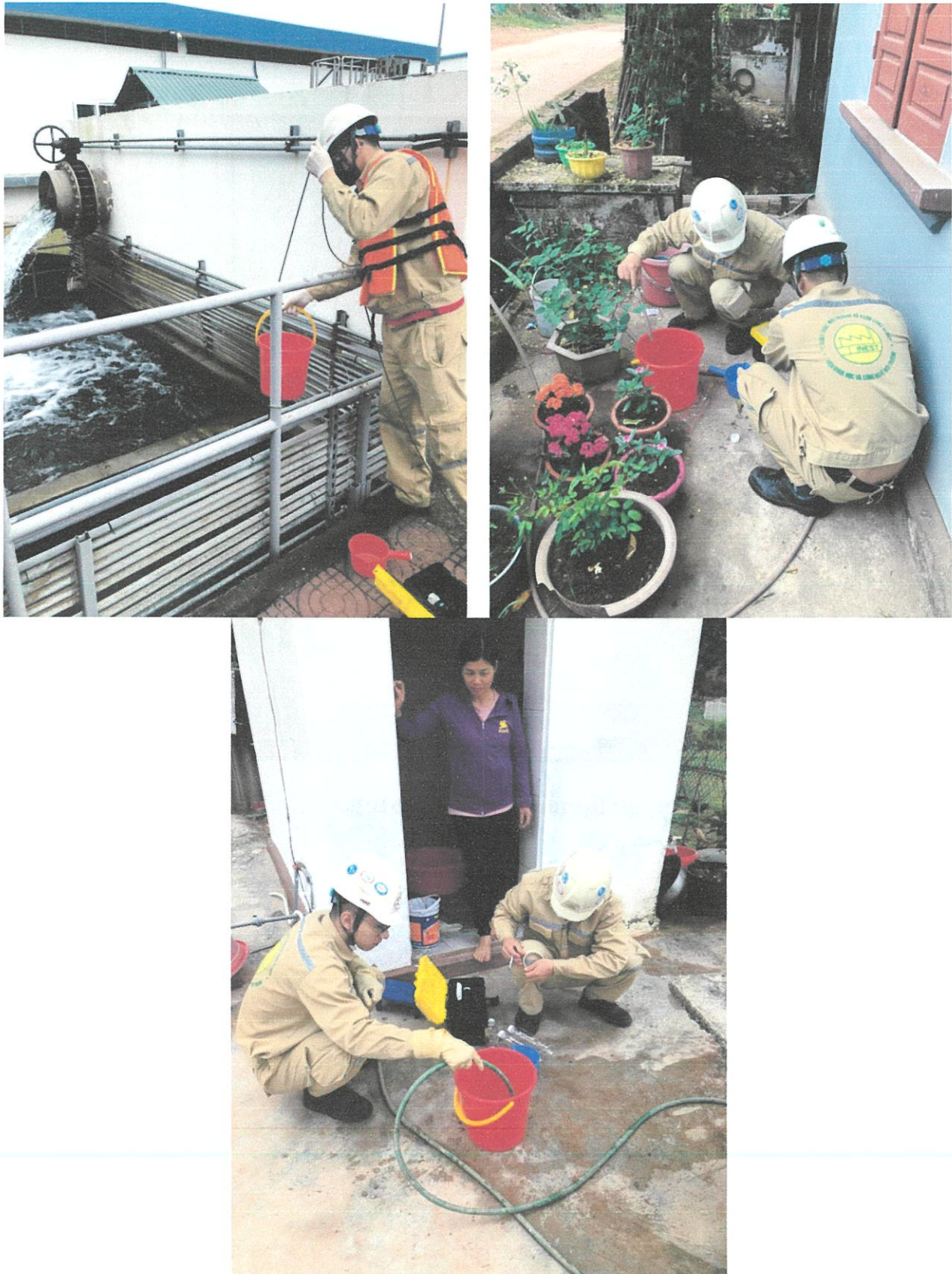
Figure 4.2. Taking surface wastewater samples, ground water samples
