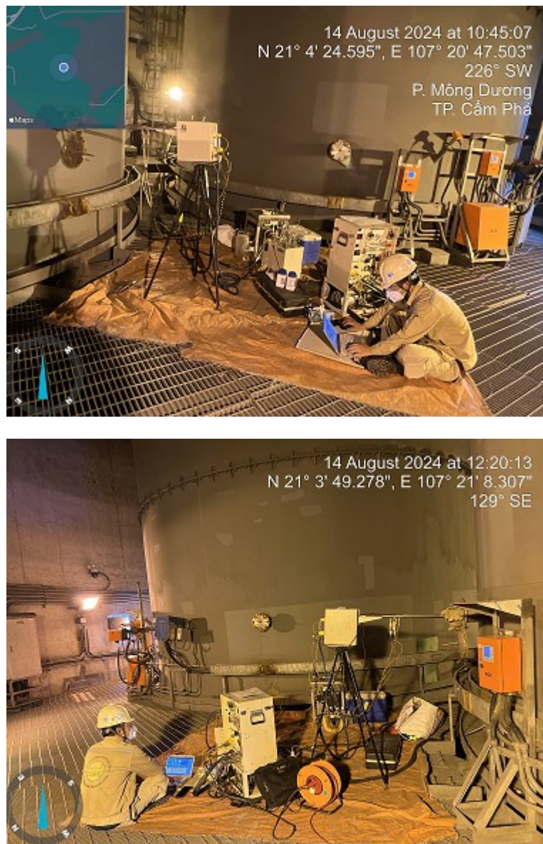
Figure 4.4. Sampling air emission in Mong Duong 2 BOT Coal Fired Power Plant
