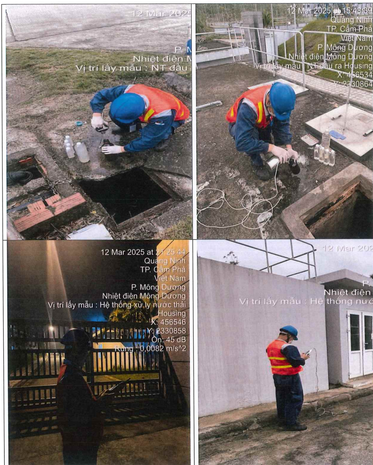
Figure 4.6. Measuring noise and vibration and taking wastewater samples - - Wastewater Treatment System at the Housing Colony
