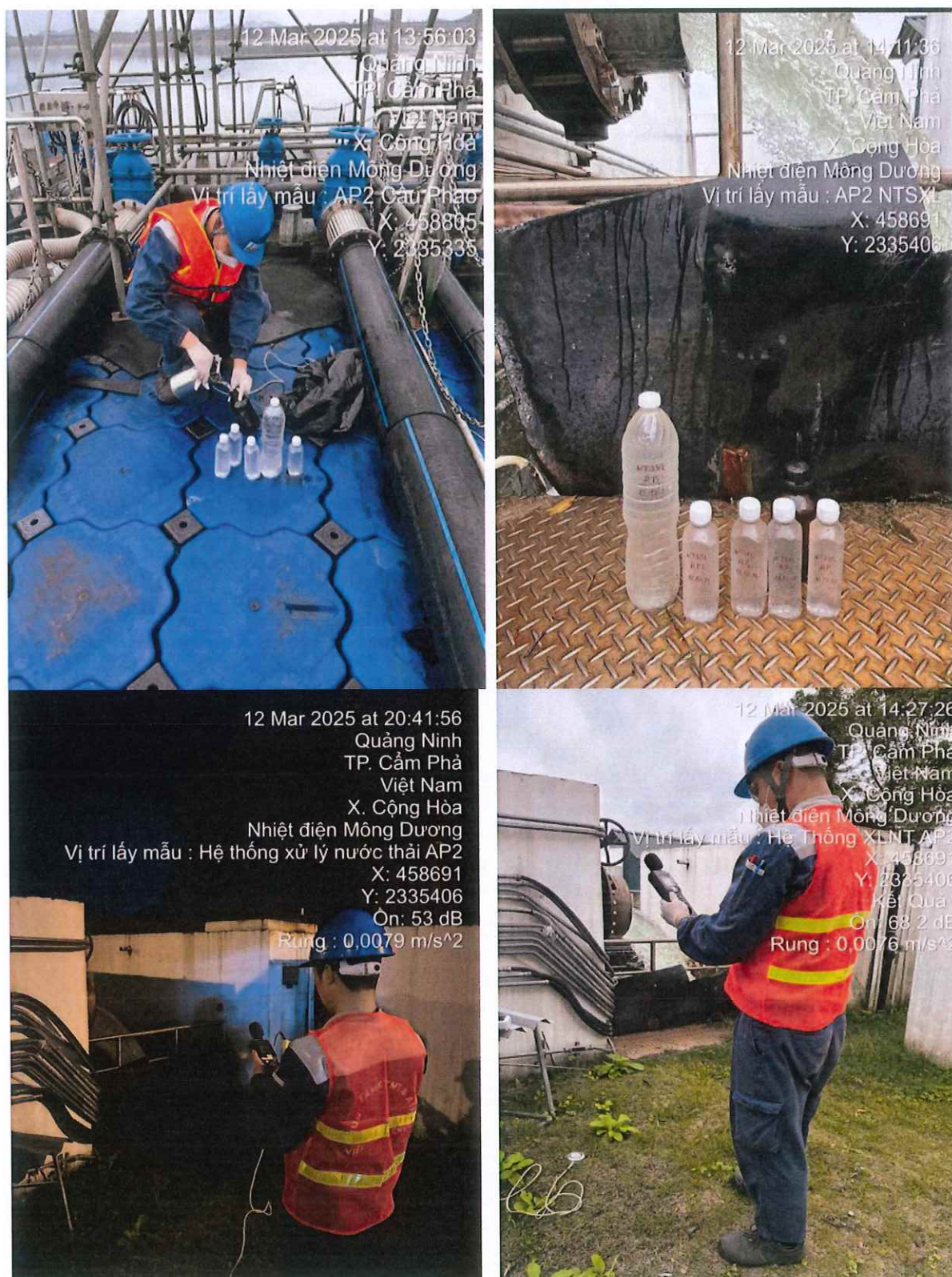
Figure 4.5. Measuring noise and vibration and taking wastewater samples - Ash Pond 2
